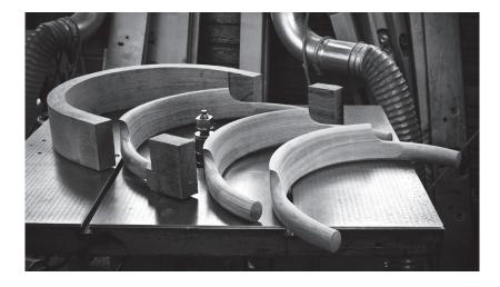
The most common and easiest way to design a more production friendly wooden chair with excellent back support is to steam bend a single length of solid wood cut from 80-100 year old trees. The semi-conditioned wood is steamed for some hours before it is bent with immense force. The final conditioning after bending takes about 3-4 months.
